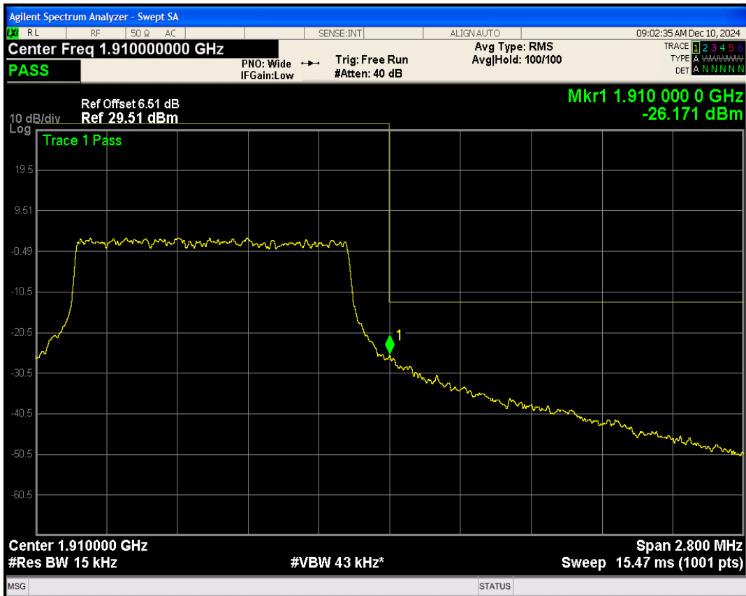
Band2 QPSK BW=3MHz Channel=18615 RB Size=15 Position=#0
