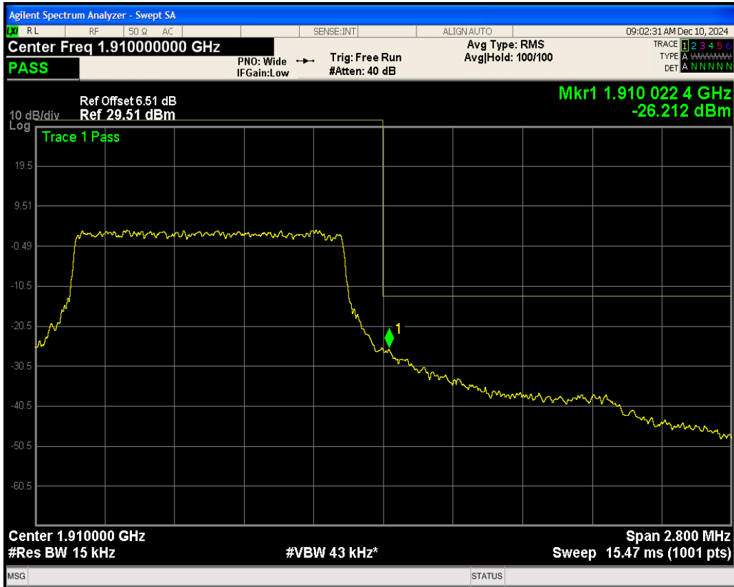
Band2 16QAM BW=1.4MHz Channel=19193 RB Size=6 Position=#0
