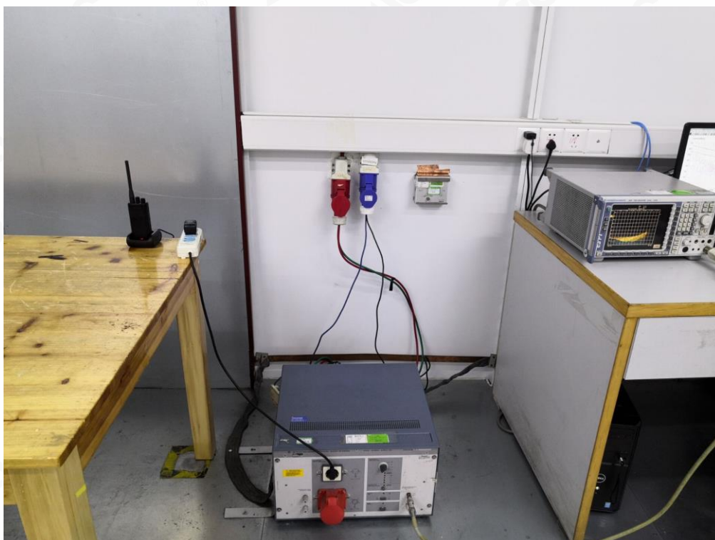
RADIATED EMISSION TEST SETUP-BELOW 1GHZ
