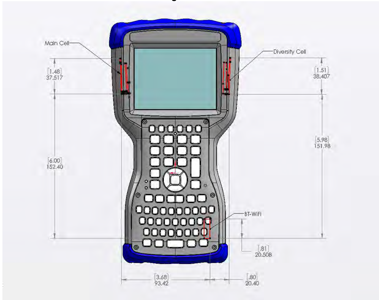
Figure 9.1 SAR Location Diagram of Antenna Distances
