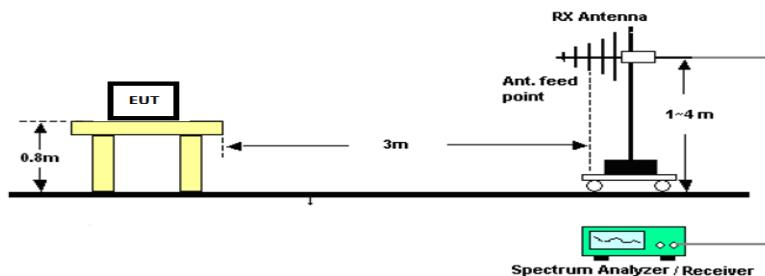
Radiated Test Setup, Above 1000 MHz
