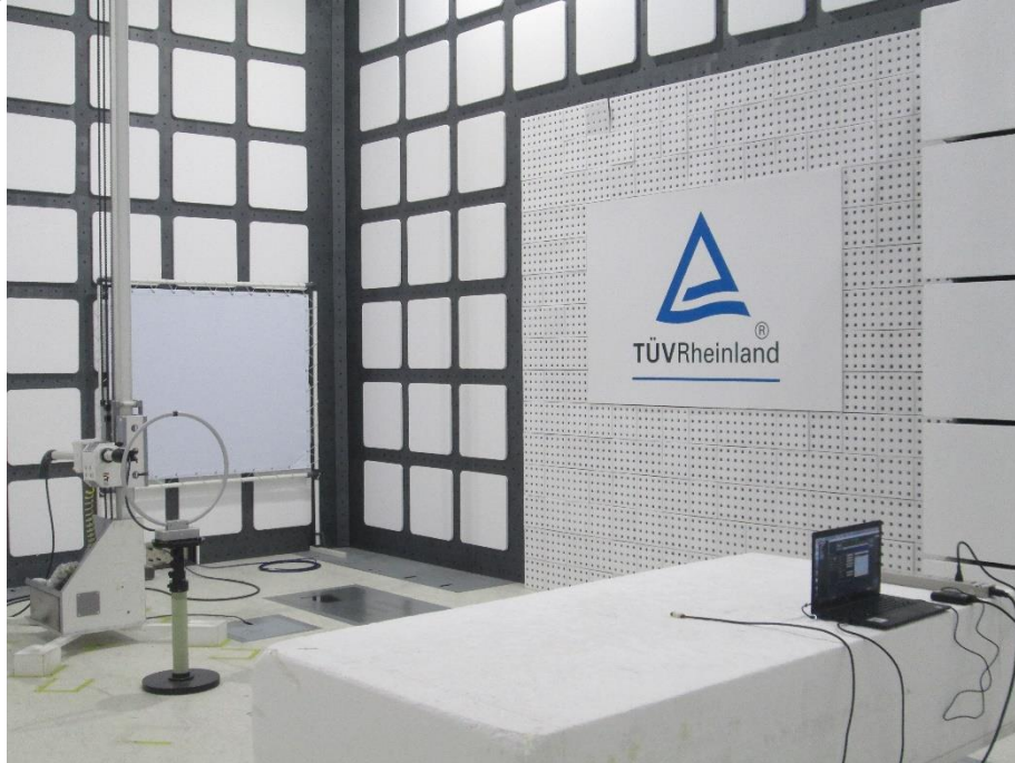
Photograph 3: Test Setup for Spurious Emissions (Back View 1)
