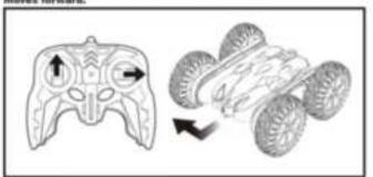
Remote control right joystick push to the left, the car moves to the left.
