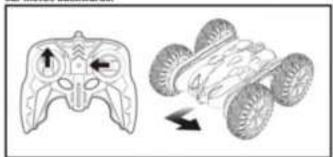
The remote control right rocker pushes to the right and the car moves to the right.
