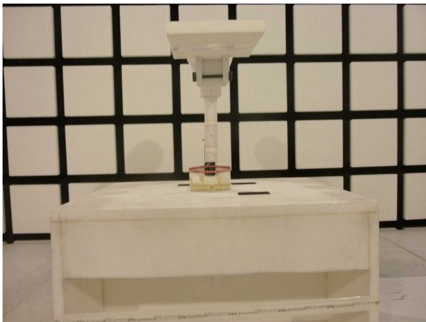
Photo 10: EUT at the anechoic chamber, loop antenna test setup
