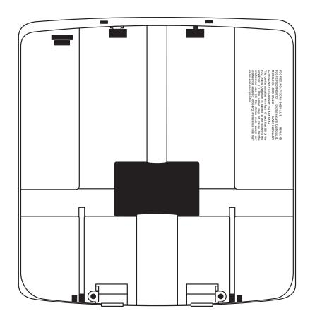
The FCC/IC labeling is to be located on the top of the rear housing of the unit as shown above. This illustration and labeling are shown 50% of the actual size.
