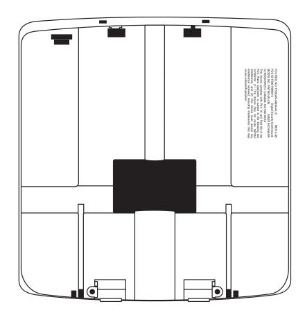
The FCC/IC labeling is to be located on the top of the rear housing of the unit as shown above. This illustration and labeling are shown 50% of the actual size.
