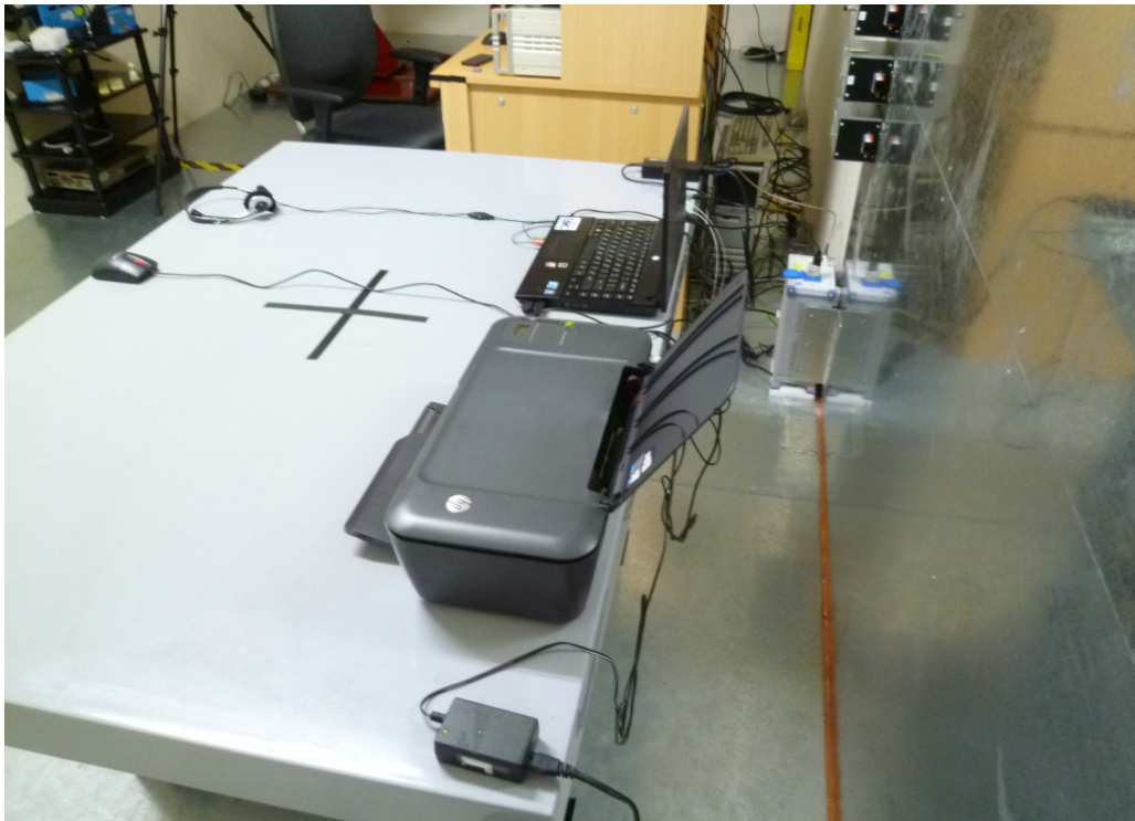
Photograph 5: Set-up for for Mains Conducted testing Back
