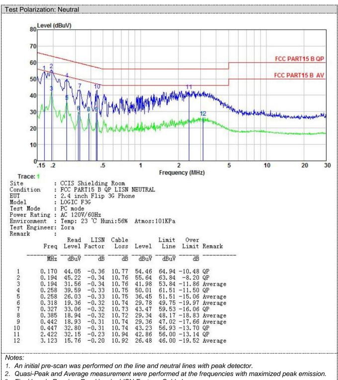
3. Final Level =Receiver Read level + LISN Factor + Cable Loss.
