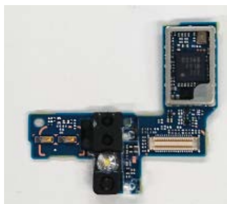
Internal Sub-PWB without Shield cases (Front-side)
