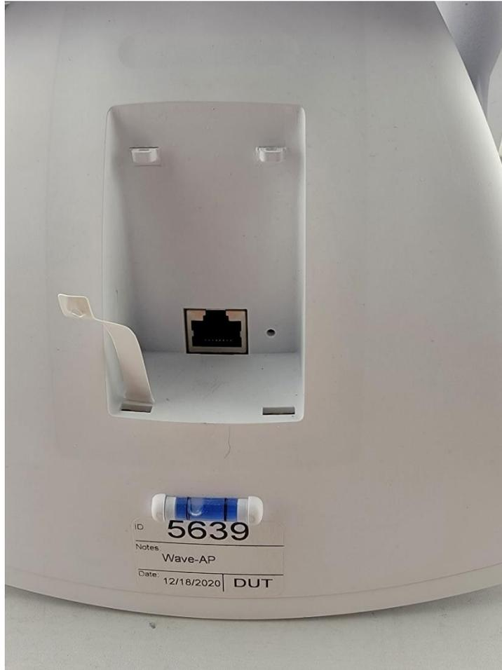
**Photograph 5: Back View of DUT Cover Removed Showing RF45 Jack**
