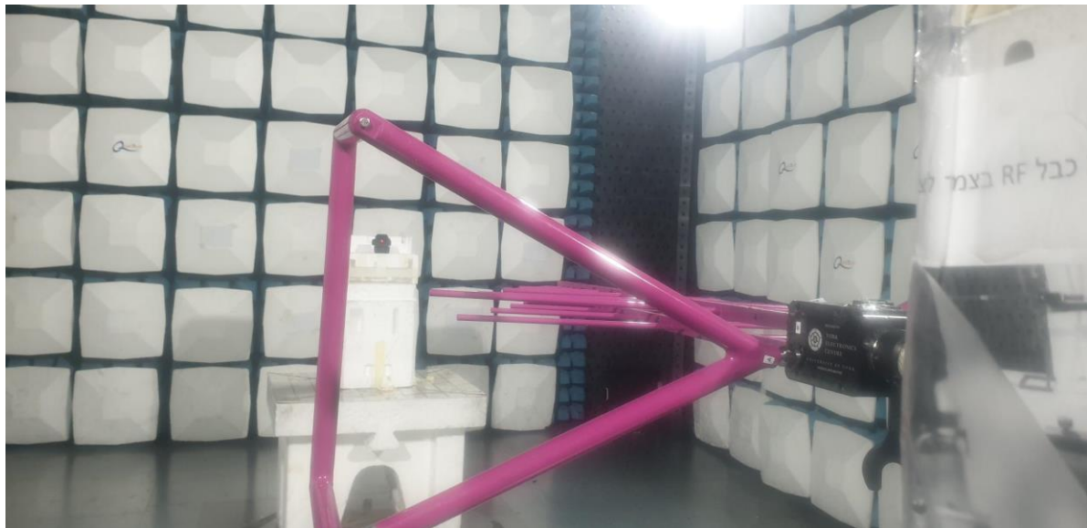
Photograph 6.2 Setup for spurious emission field strength measurements from 30 to 1000 MHz
