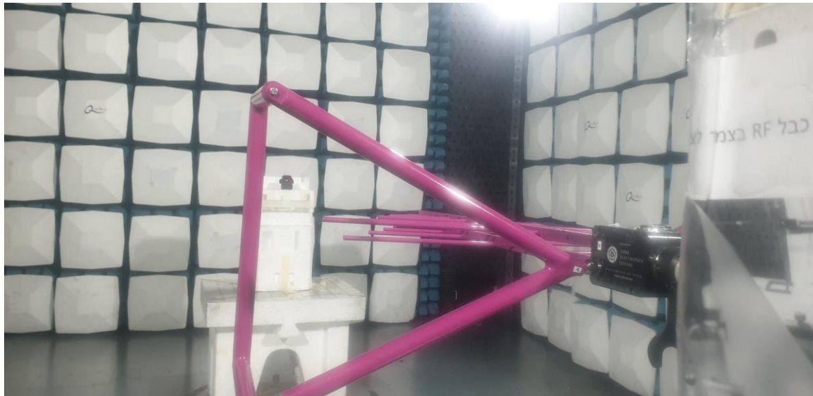
Photograph 5.1 Setup for carrier field strength measurements
