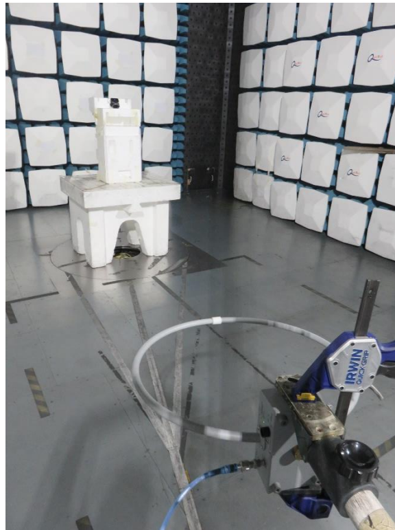
Photograph 6.1 Setup for spurious emission field strength measurements below 30 MHz
