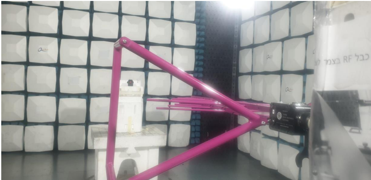
Photograph 4.1 Setup for carrier field strength measurements
