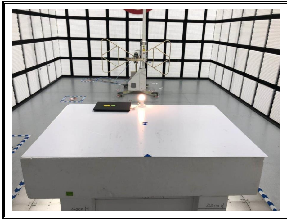
RADIATED RF MEASUREMENT SETUP (Below 30MHz)
