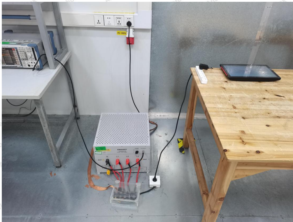
Photo of Conducted Emission Measurement
