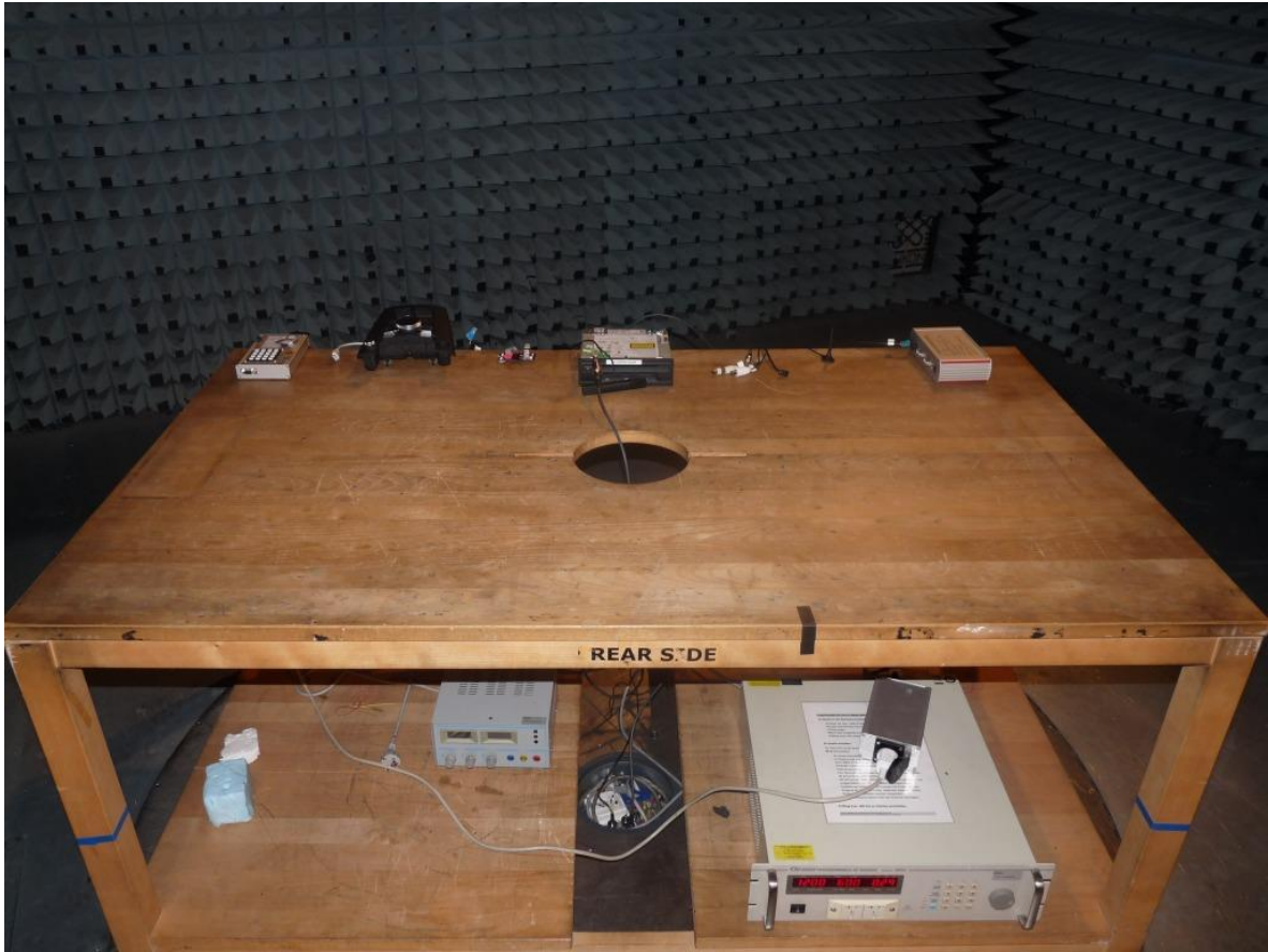
Photo 2: Test setup for radiated measurements, front view (Enclosure, semi-anechoic chamber, 30 MHz to 1 GHz, intentional radiator §15)
