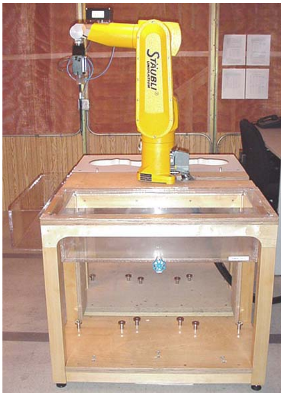
DASY4 SAR Measurement System with validation phantom
