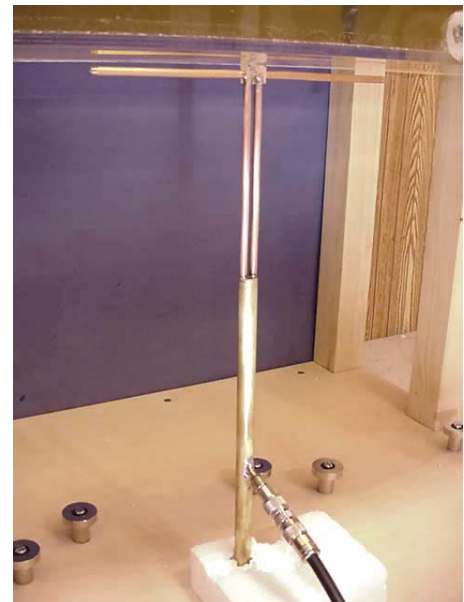
450MHz System Check Setup
