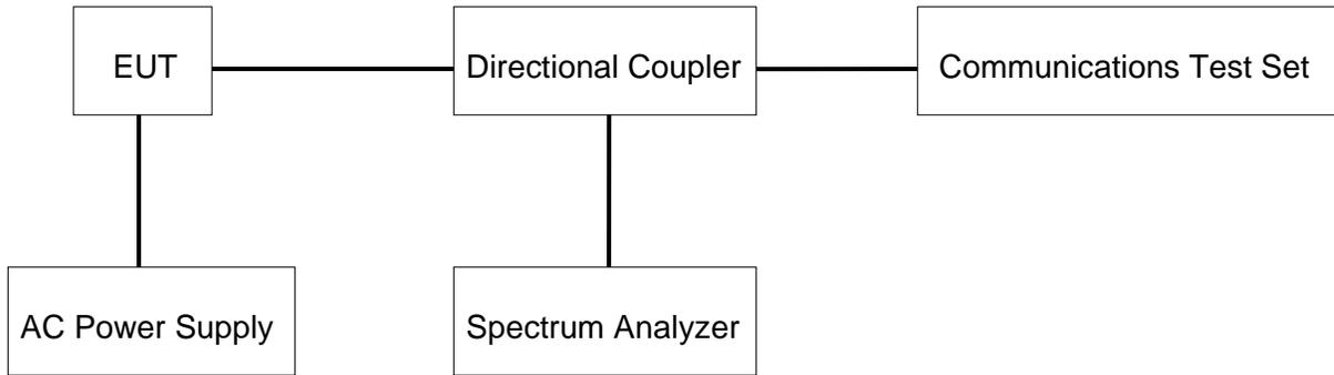
**RADIATED TEST SETUP**
