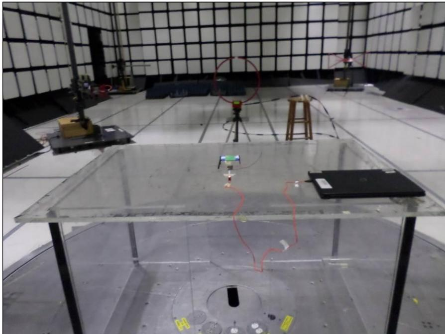
**Photograph 2. Radiated Emissions, 0.009 – 1.250 MHz, Rear View**
