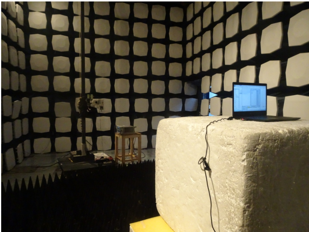
Picture 1 Radiated Emission Test Setup
