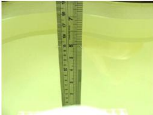
Fig 6.1 Photo of Liquid Height for Head SAR
