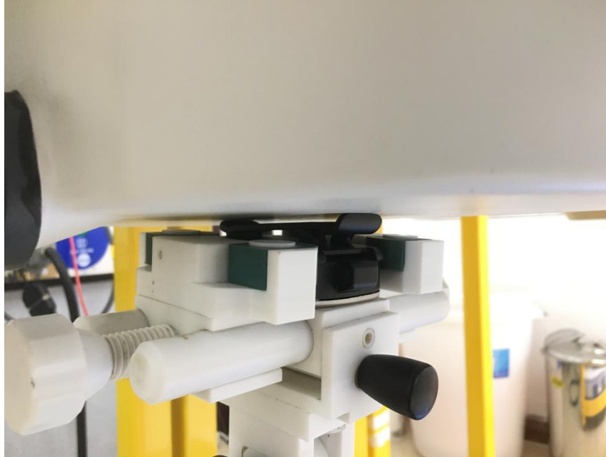
Body worn _ Back with Clip (Test distance: 0mm, Thickness of DUT: 16mm)
