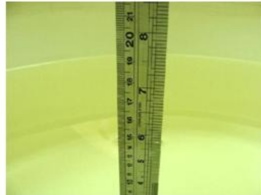
Fig 6.2 Photo of Liquid Height for Body SAR
