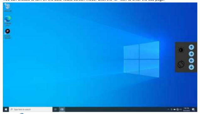
Click the  $\infty$  icon to switch between automatic and manual rotate modes. In auto-rotate mode, the screen automatically rotates depending on the device's orientation. To select the manual-rotate mode, please use the right button to complete the setting.
