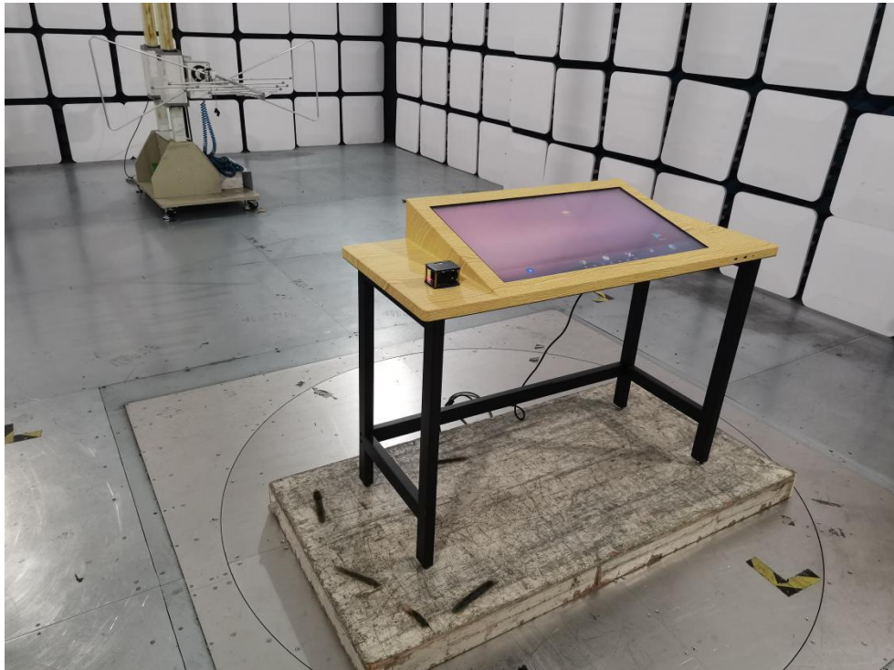
Photo of Radiation Emission Test
