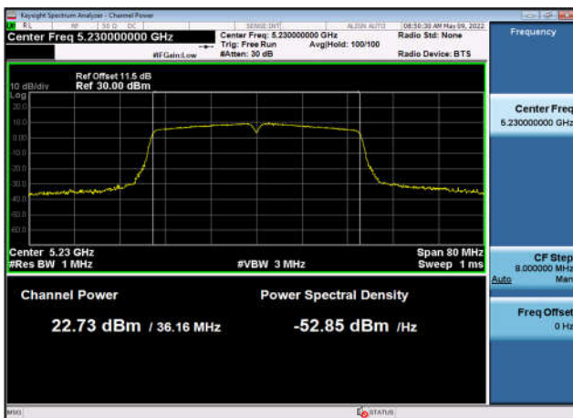
U-NII-1 Output Power-802.11ax(40MHz) ,5230MHz,Ant2
