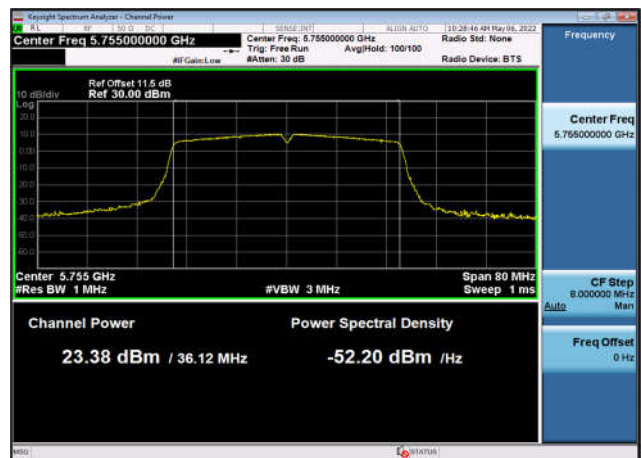
U-NII-3 Output Power-802.11ax(40MHz) ,5755MHz,Ant2
