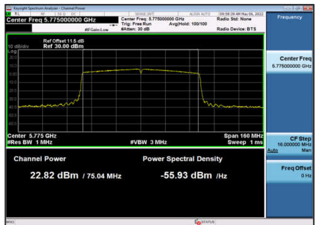
U-NII-3 Output Power-802.11ax(80MHz) ,5775MHz,Ant1
