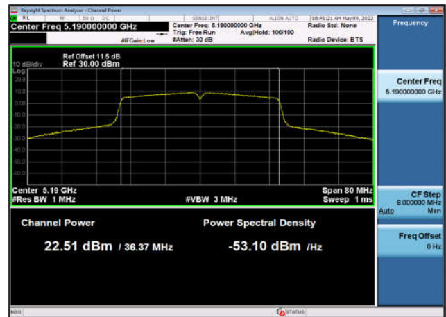
U-NII-1 Output Power-802.11ax(80MHz) ,5210MHz,Ant2
