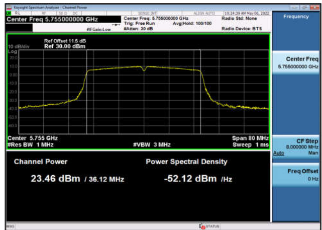
U-NII-3 Output Power-802.11ax(80MHz) ,5775MHz,Ant1
