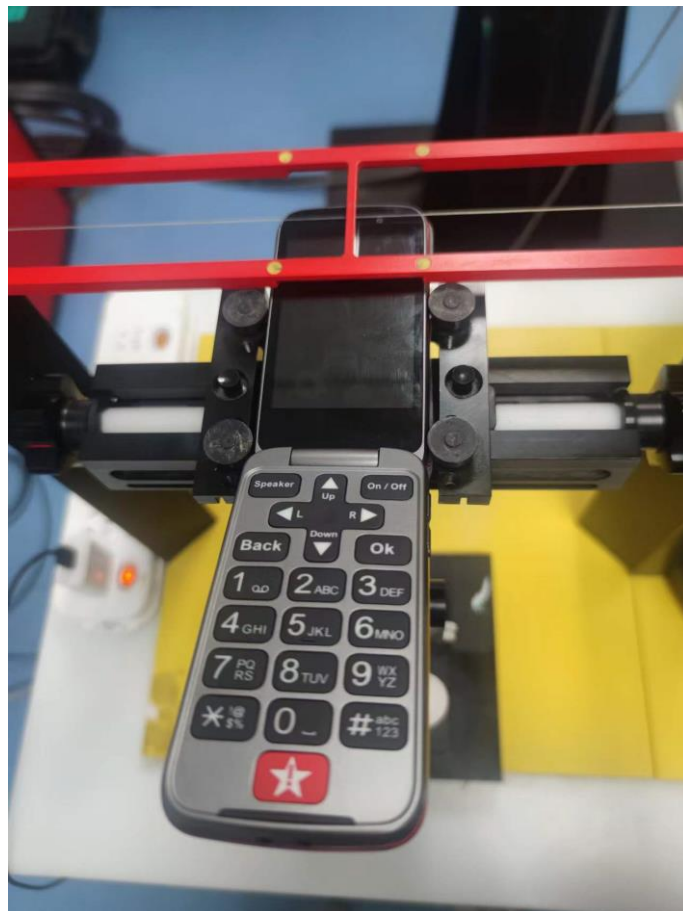
Picture 2: EUT Positioning for RF/T-coil
