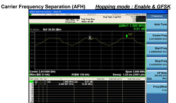
Carrier Frequency Separation (AFH) <u>Hopping mode : Enable & π/4DQPSK</u>
