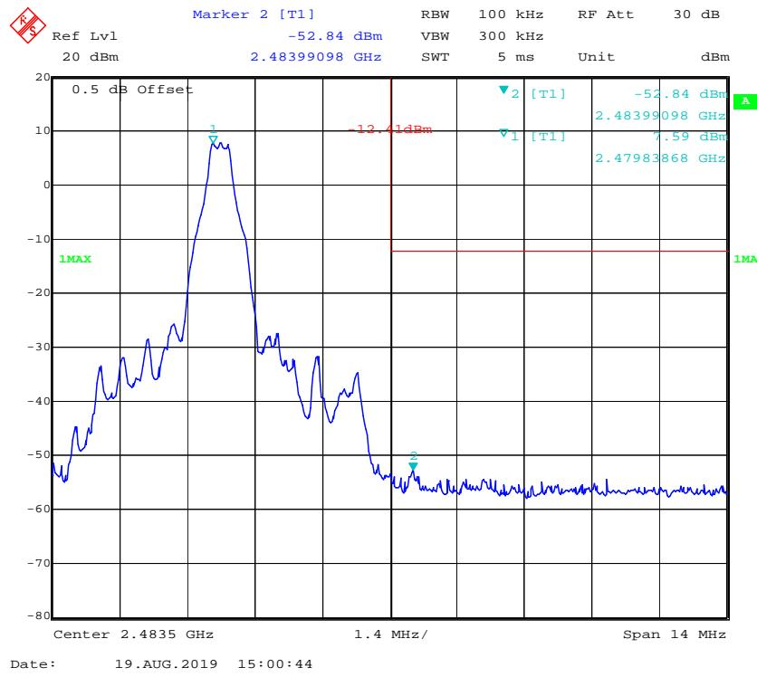
*EDR Mode ( $\pi/4$ -DQPSK):***Band Edge, Left Side**
