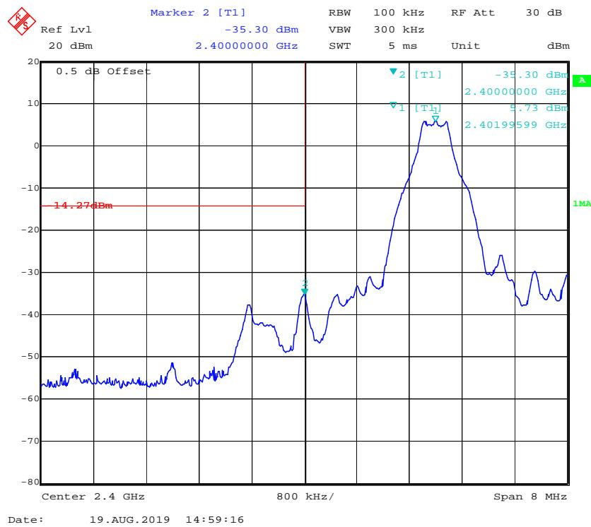
**Band Edge, Right Side**
