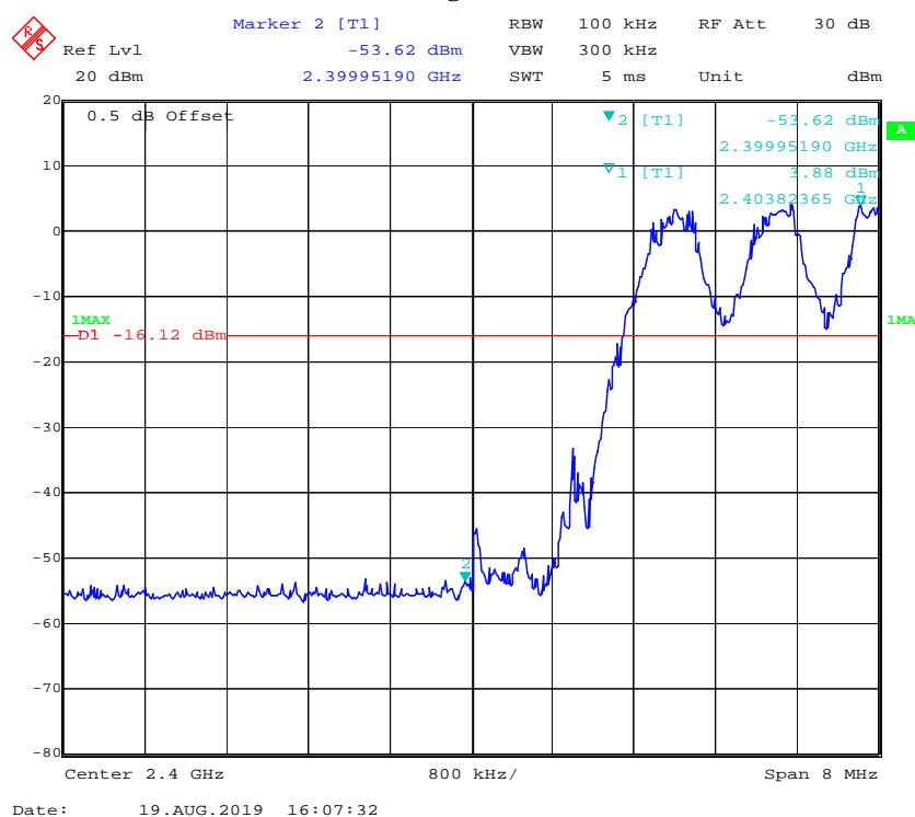
**Band Edge, Right Side**
