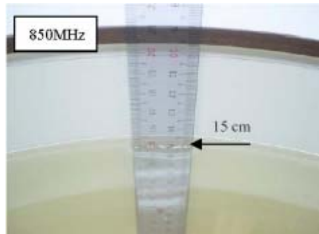
Fig.3 Photograph of the Tissue Simulant Liquid depth 15cm for Body-Worn
