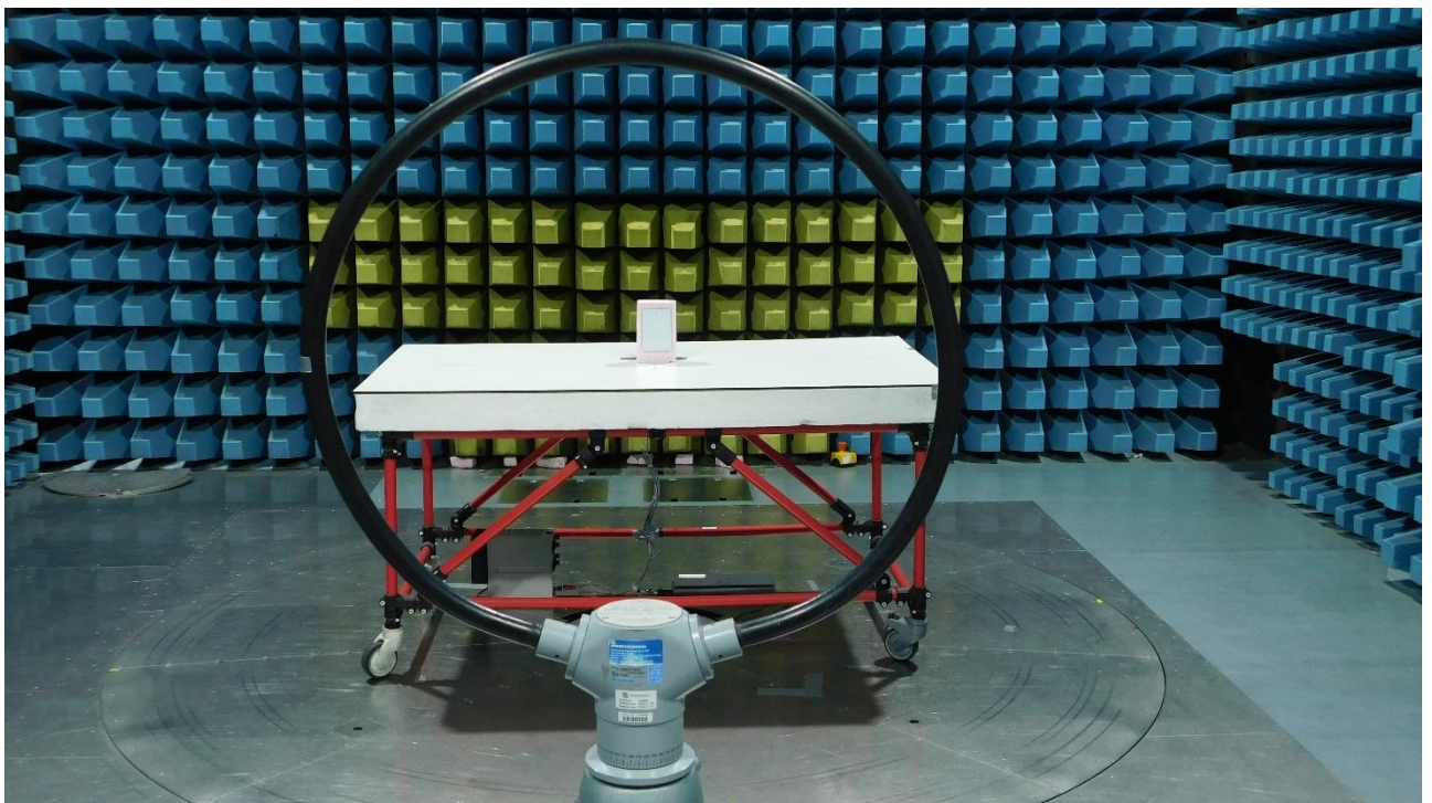
Picture 11: SAC, test setup radiated emission test 9 kHz - 30 MHz (rear view)
