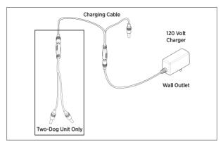
The Dogtra 280C uses a lithium polymer battery. Recharge the unit if the indicator light is red or does not come on, the transmitter LCD shows only 1 bar on the indicator, or the system will not stay on when any button is pressed.
