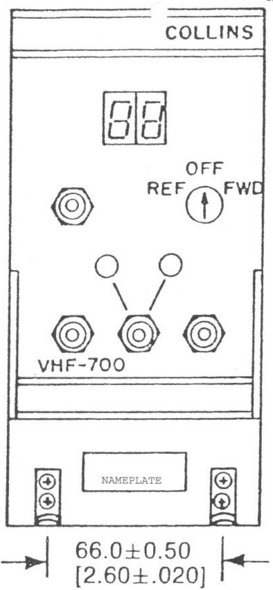
$\underline{\text{Note}}$ : This drawing is included to show the relative size and placement of the nameplate for the VHF-700A. See the previous page for a drawing of the actual nameplate.
