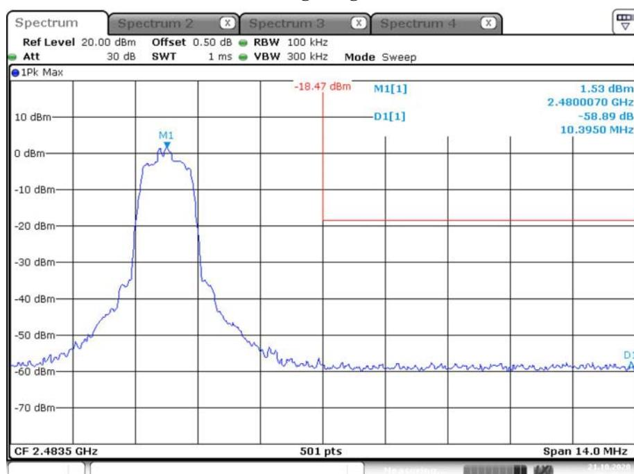
*EDR Mode (8DPSK)***Band Edge, Left Side**
