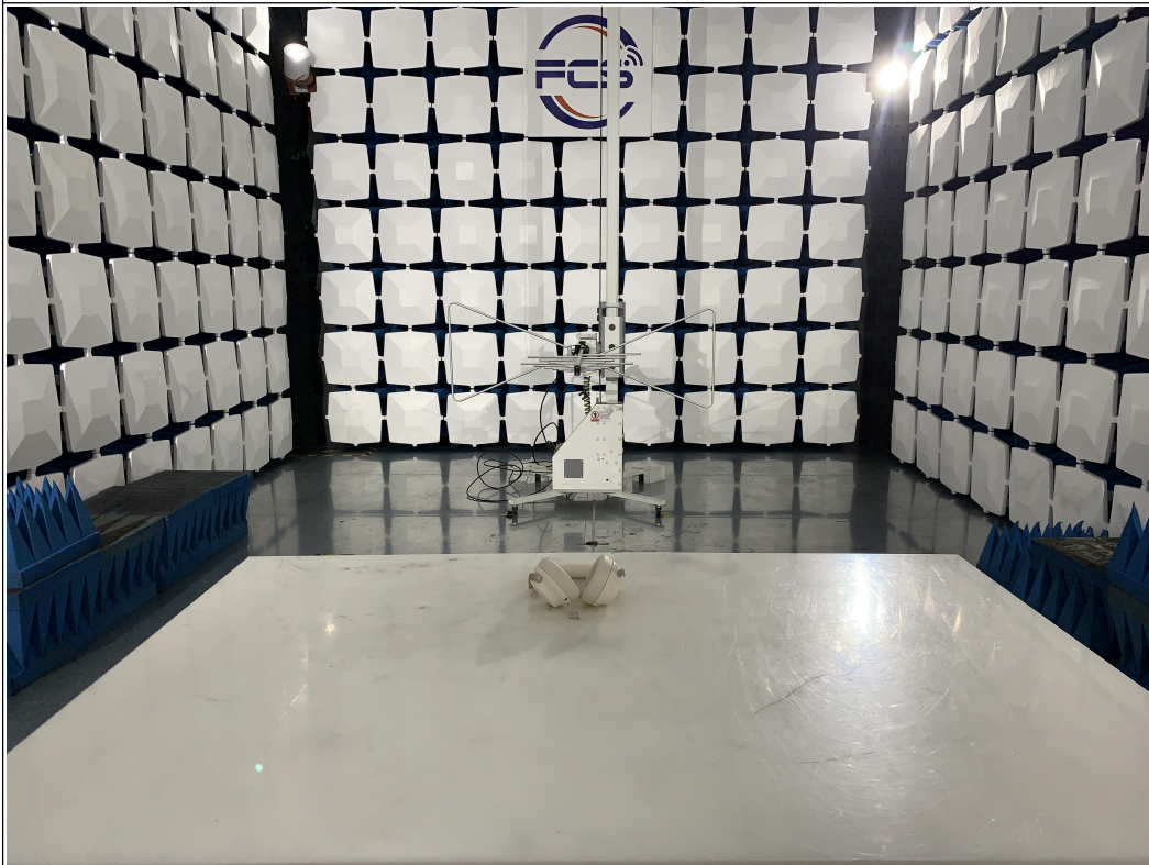
Above 1GHz for radiated emission test setup
