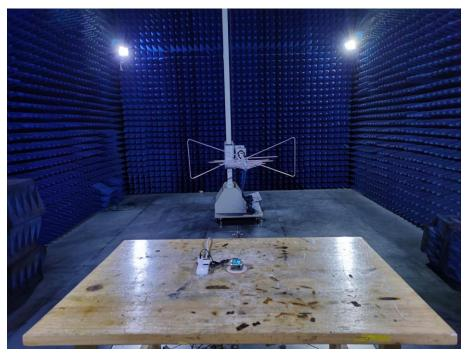
3. Photo of Radiated Emission Measurement 30MHz - 1GHz
