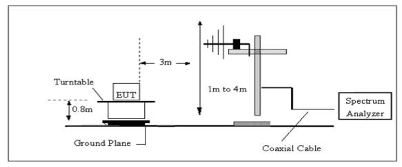
(A) Radiated Emission Test-Up Frequency 30MHz~1GHz
