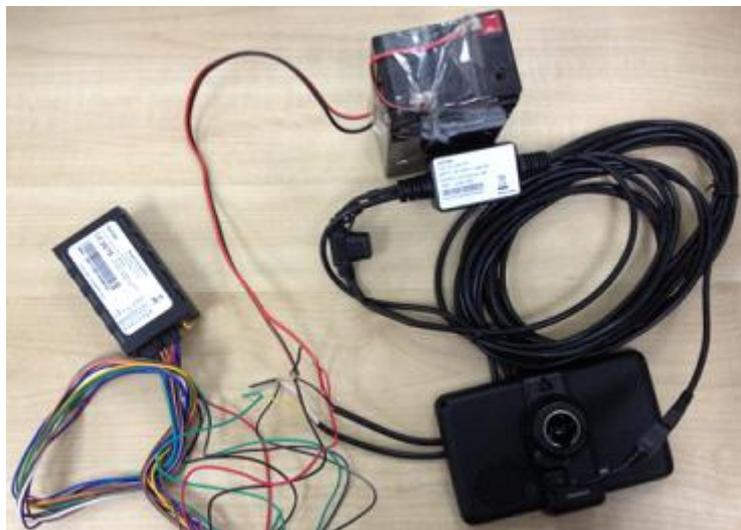
Figure 18. GV300W Connection with Garmin GPS Set
