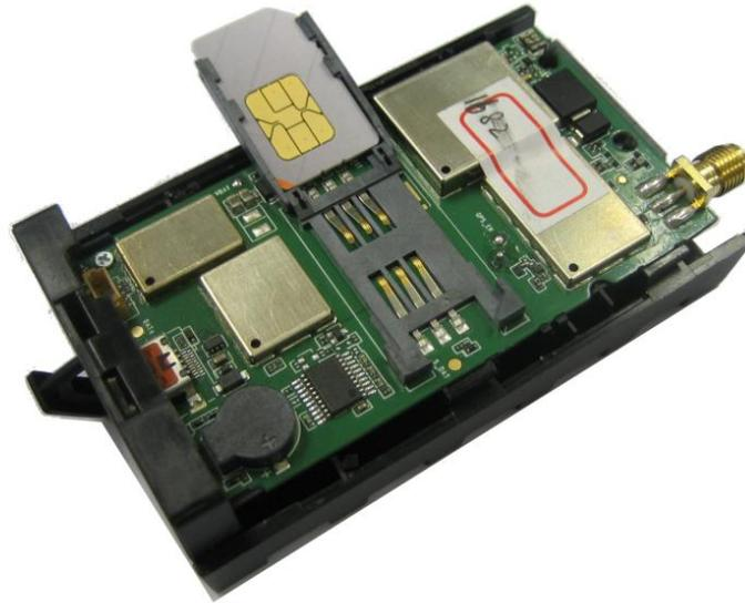
Figure 5. SIM Card Installation
