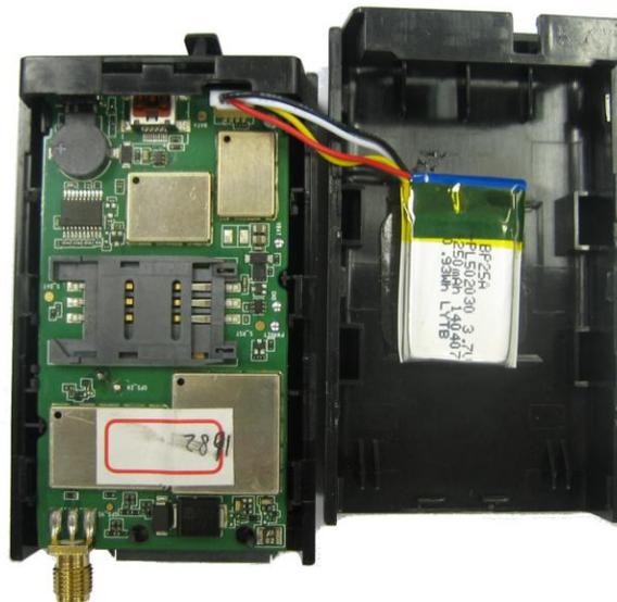
Figure 6. Backup Battery Installation
