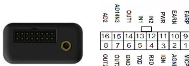
Figure 2. The 16 PIN Connector on the GV300W
