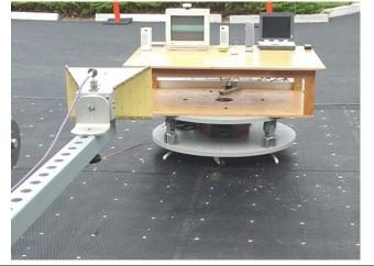
Photograph E-3 - Front of Radiated Emission Configuration
