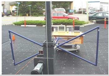
Photograph F-3 - Front of Radiated Emission Configuration
