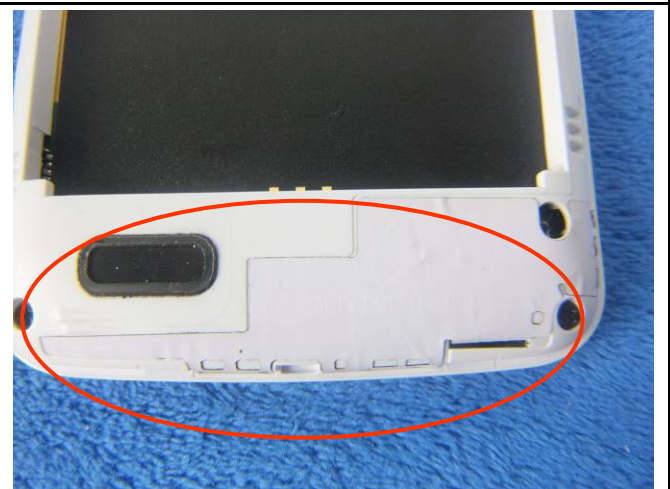
GSM/PCS/UMTS-FDD/LTE - Antenna View
