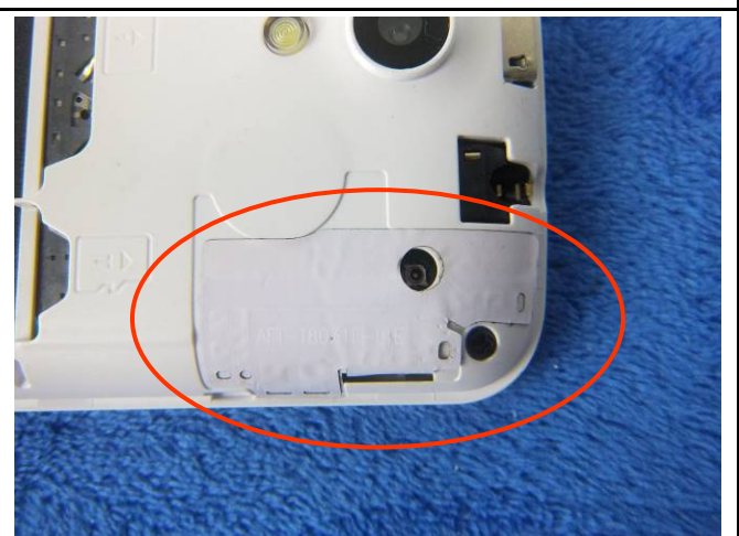
LTE - Antenna View
