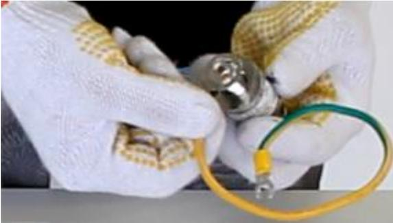
2. Connect one end of the GPS RF cable to the GPS lightning arrester, as shown in Figure 4-4.
