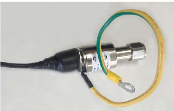
4. Connect the GPS RF cable to the GPS antenna lightning arrestor. It is necessary for the GPS antenna interfaces to be weatherproofed. Refer to 3.5 Weatherproof Protection for more detail. The connection is complete shown in Figure 4-6.
