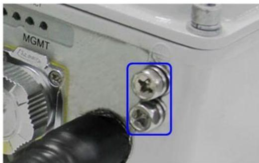
1. Unscrew one grounding screw, connect the GPS lightning arrestor grounding cable
