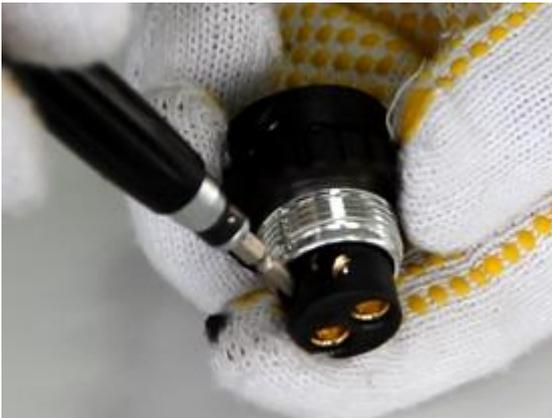
4. Insert the red power cable (48V) into terminal A, and insert the black power cable (0V) into terminal B, as shown in Figure 4-14.
