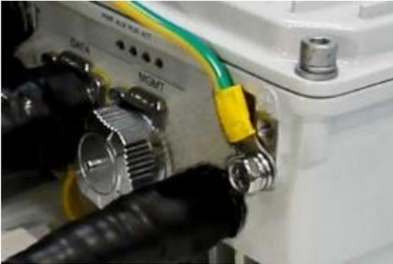
2. Unscrew another grounding screw, connect one end of the ground cable to the grounding screw of the device, as shown in Figure 4-18.
