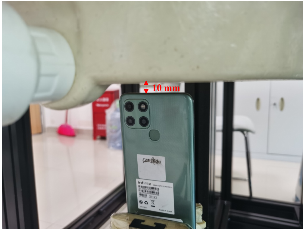
Body Top Setup Photo (10mm)
