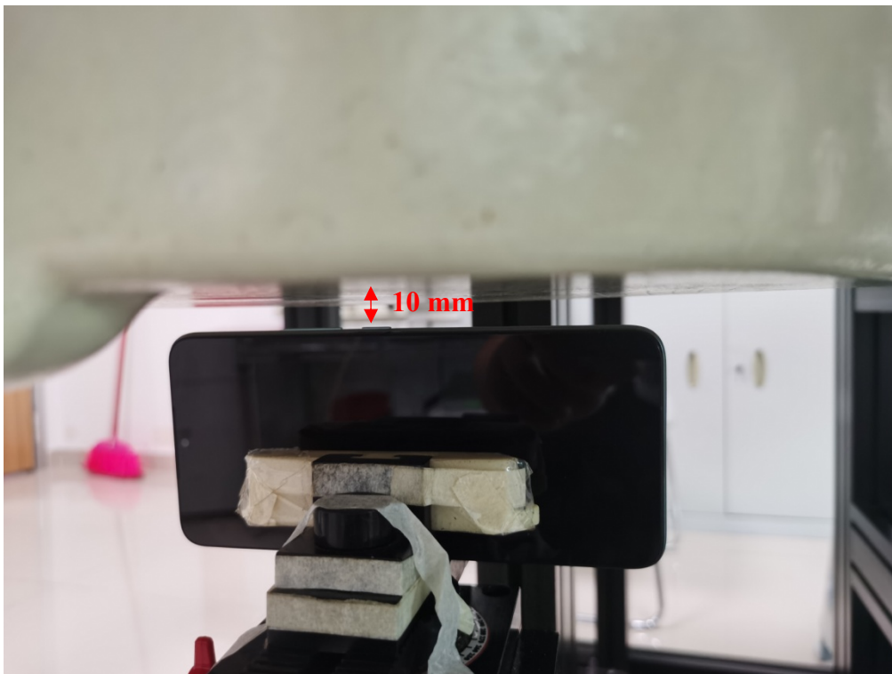
Body Right Setup Photo (10mm)
