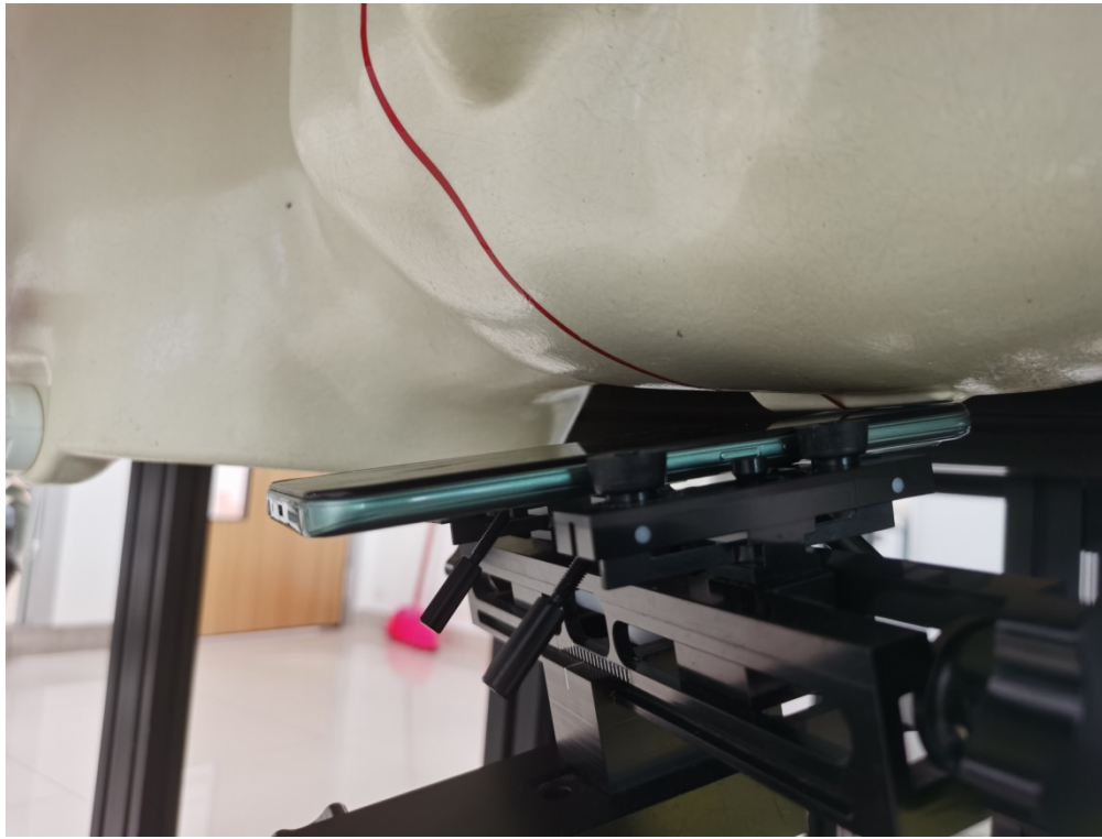
Head Right Cheek Setup Photo
