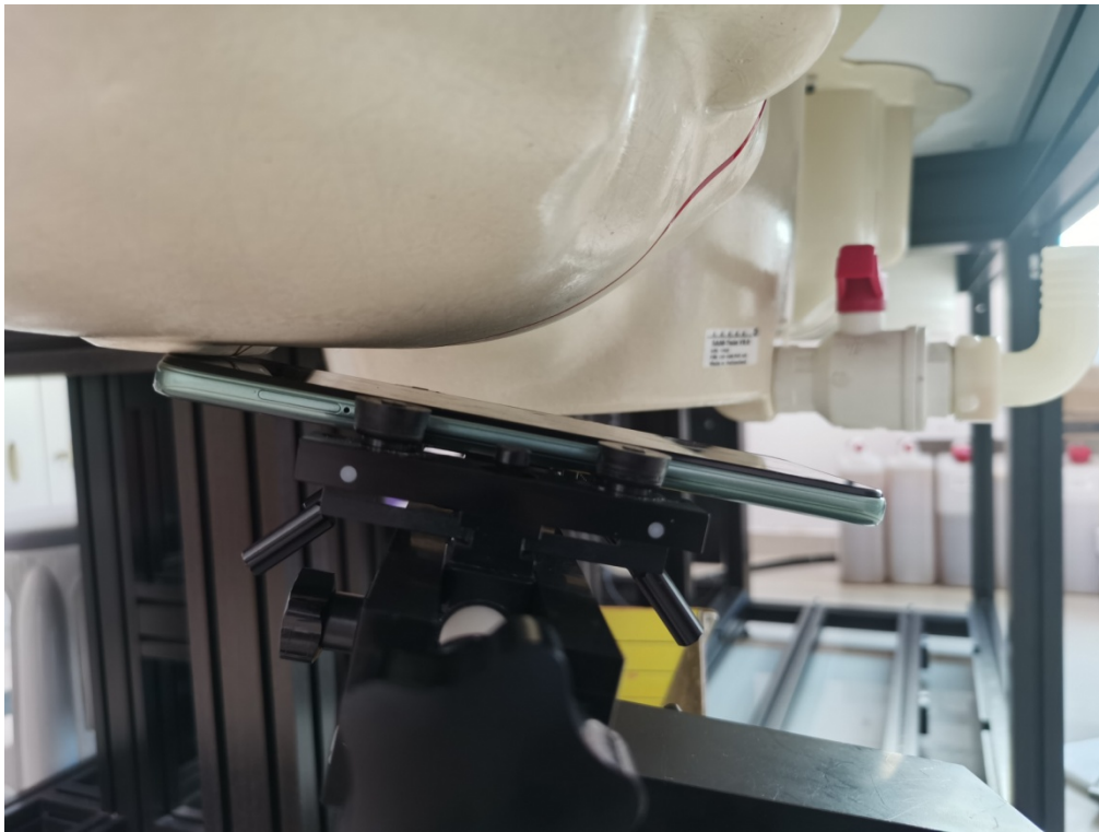
Head Right Tilt Setup Photo
