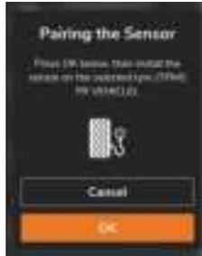
7. Install the pressure sensor on the same selected tyre. Refer to the section **Installing SmartPressure Sensors**.
