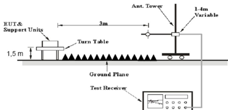
The radiated emissions were performed in the 3 meters distance, using the setup accordance with the ANSI C63.10-2013. The specification used was the FCC 15.209, and FCC 15.247 limits.
