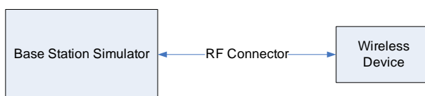
Figure 9-1 Power Measurement Setup
