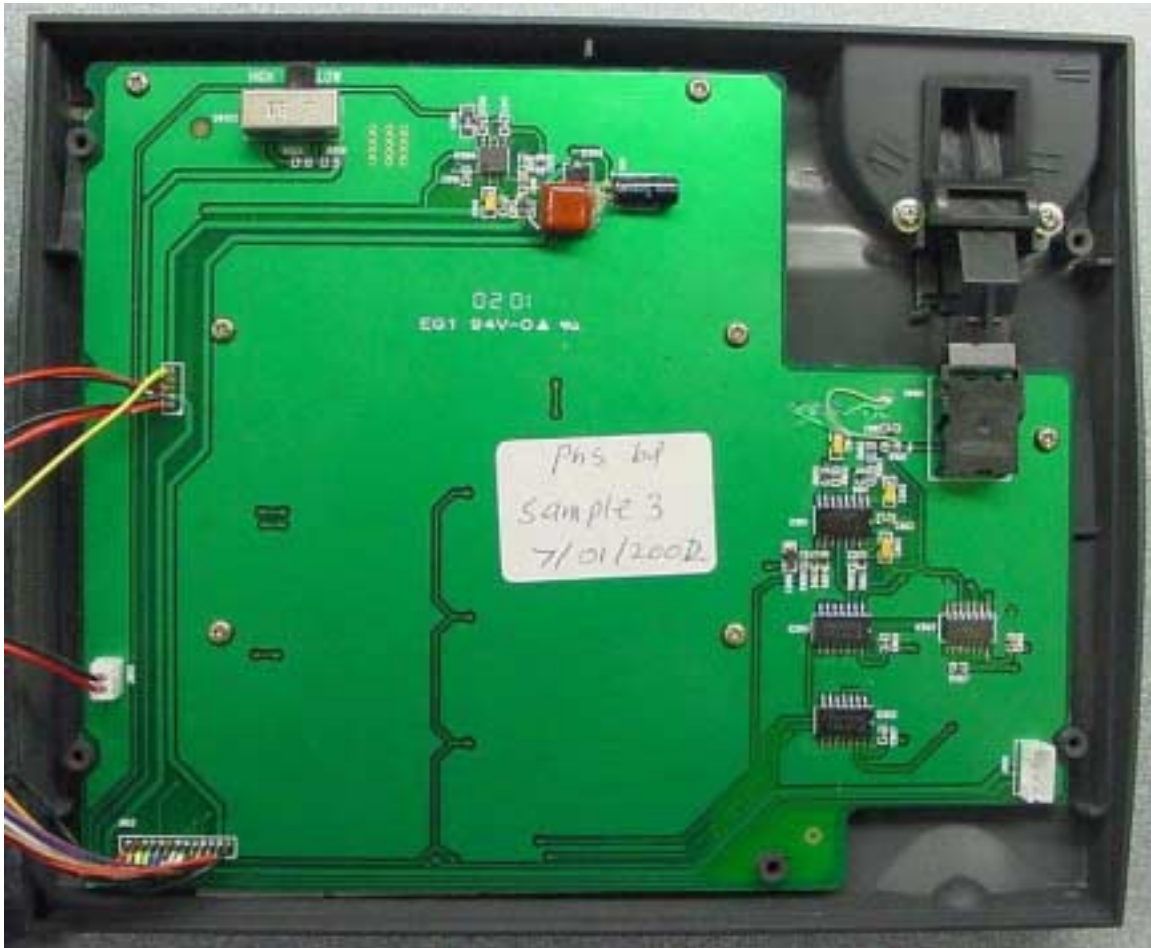
PHOTOGRAPH 15: INSIDE TOP CASE WITH KEYPAD PCB ATTACHED
