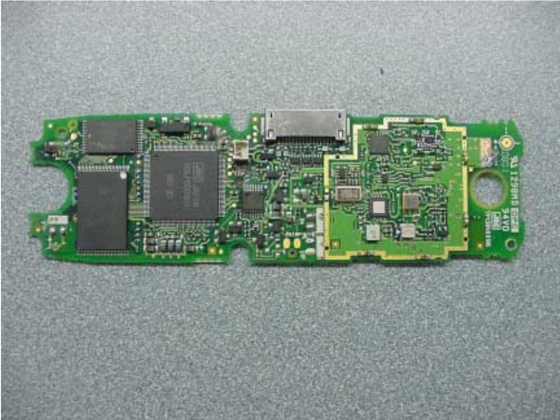
PHOTOGRAPH 45: COMPONENT SIDE OF RF PCB WITH SHIELDS REMOVED
