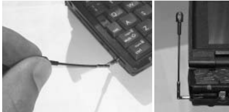
Figure 3-8: Pivoting the AirCard 710 Antenna at the Hinge
