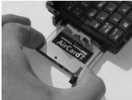
Figure 3-18: Removing the AirCard 710 PC Card From Its Slot
