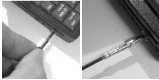
Figure 3-7: Extending the AirCard 710 Antenna Until It Clicks Into Place
