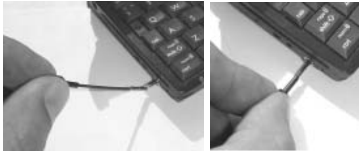
Figure 3-16: Retracting the AirCard 710 Antenna
