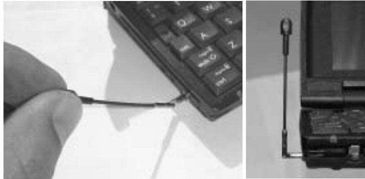
Figure 3-11: Pivoting the AirCard 710 Antenna at the Hinge
