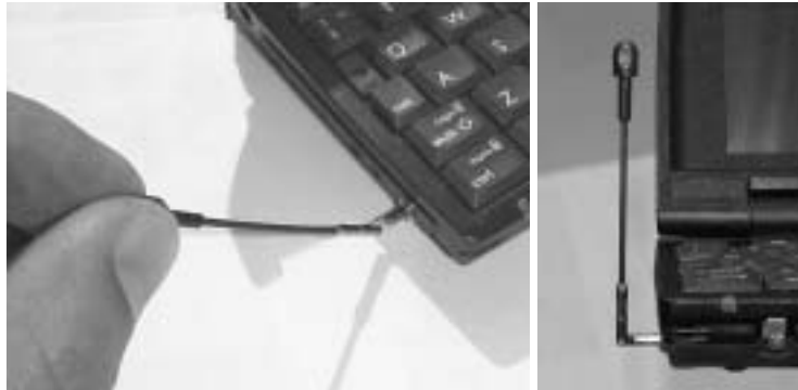
Figure 3-5: Pivoting the AirCard 710 Antenna at the Hinge
