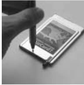
Figure 2-4: Positioning a Pen to Eject the SIM Card
