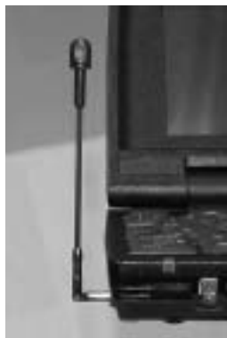
Figure 2-7: (Left) Proper Positioning of the AirCard 710 Antenna
