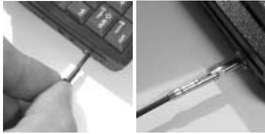
Figure 3-4: Extending the AirCard 710 Antenna Until It Clicks Into Place
