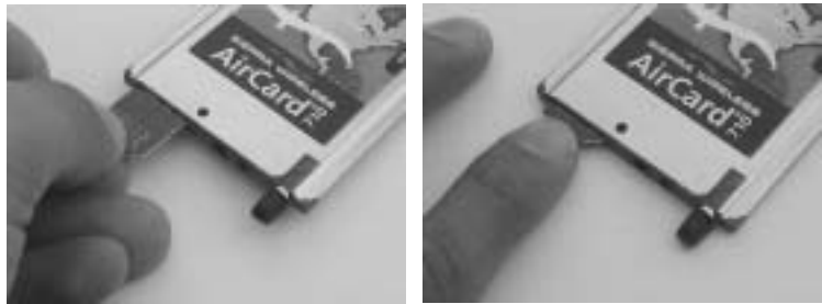
Figure 2-2: Inserting the SIM Card Into the AirCard 710 SIM Card Slot
