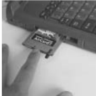
Figure 2-8: Inserting the AirCard 710 Wireless Network Card
