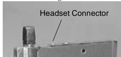
Figure 6-1: Location of the AirCard 710 Headset Connector
