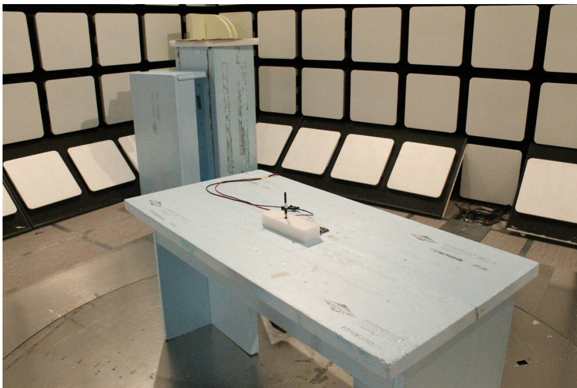
Photograph 3. EUT on table < 1GHz
