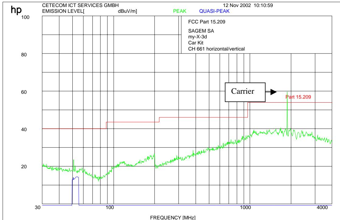
**f < 1 GHz : RBW/VBW: 100 kHz****f ≥ 1GHz : RBW 1 MHz /VBW: 10 Hz (Average)****Carrier suppressed with a rejection filter****REFERENCE NUMBER(S) OF TEST EQUIPMENT USED**
