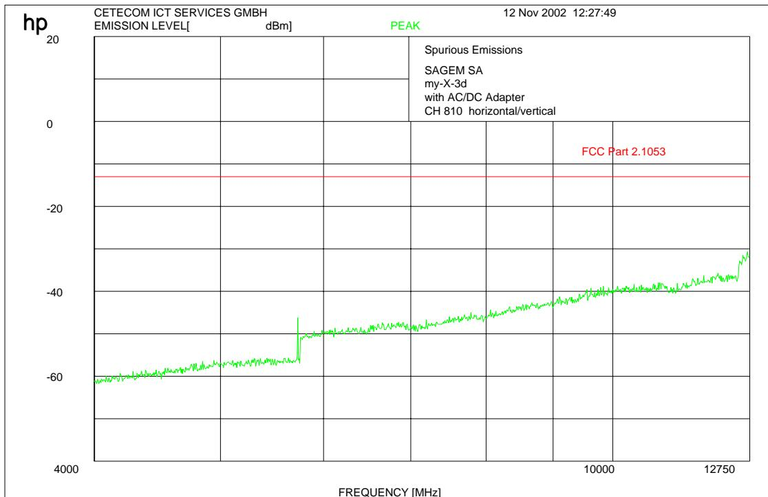
**f < 1 GHz : RBW/VBW: 100 kHz****f ≥ 1GHz : RBW/VBW 1 MHz****REFERENCE NUMBER(S) OF TEST EQUIPMENT USED**
