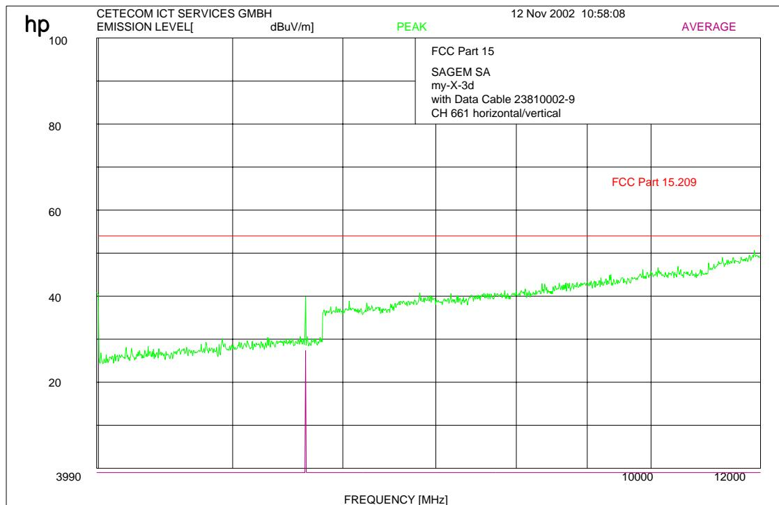
**f < 1 GHz : RBW/VBW: 100 kHz****f ≥ 1GHz : RBW 1 MHz /VBW: 10 Hz (Average)****REFERENCE NUMBER(S) OF TEST EQUIPMENT USED**
