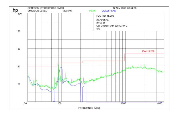
$f < 1 \; GHz : RBW/VBW : 100 \; kHz \qquad \qquad f \geq 1 GHz : RBW \; 1 \; MHz \; /VBW : 10 \; Hz \; (Average)$
