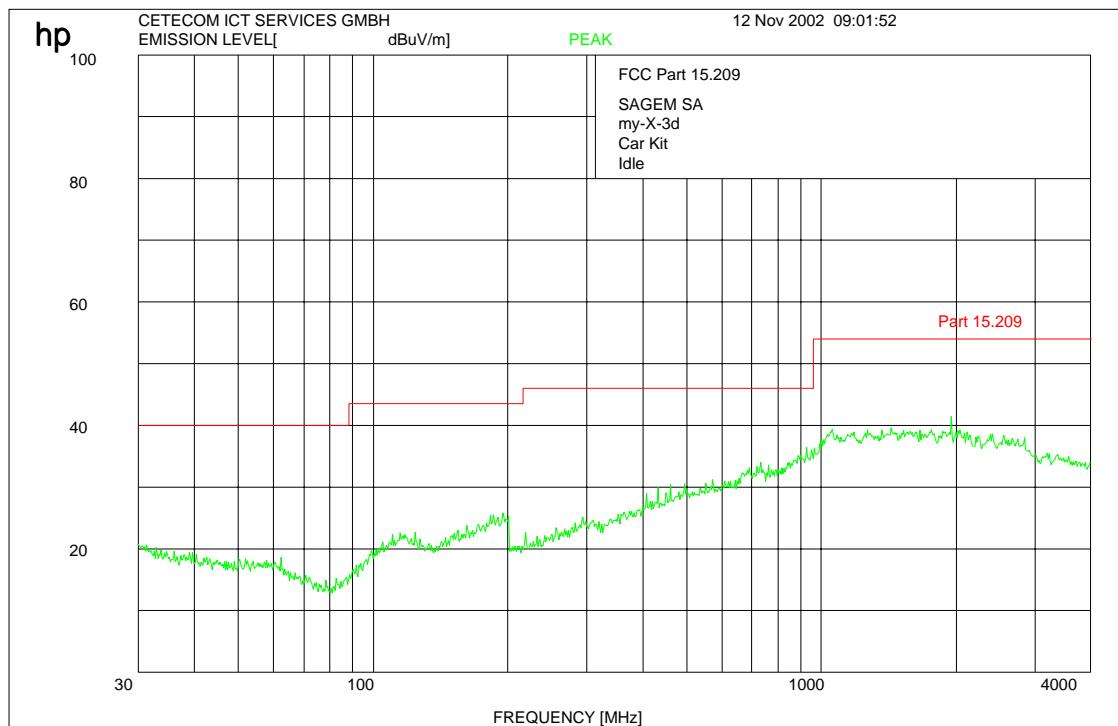
$f < 1 \text{ GHz}$  : RBW/VBW: 100 kHz $f \geq 1 \text{ GHz}$  : RBW 1 MHz /VBW: 10 Hz (Average)
