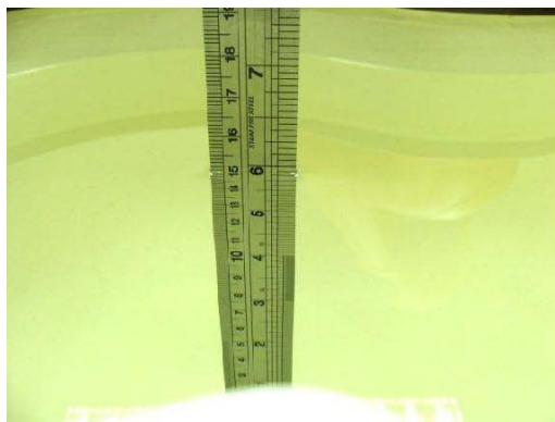
Fig 7.1 Photo of Liquid Height for Head SAR
