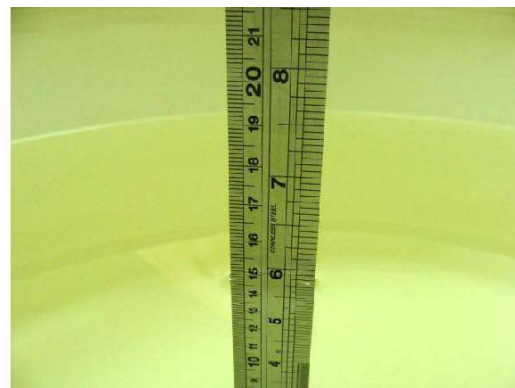
Fig 7.2 Photo of Liquid Height for Body SAR
