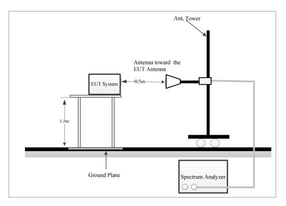
The radiated emission tests were performed in the 3 meters chamber test site, using the setup accordance with the ANSI C63.26-2015. The specification used was the FCC 95.3379 limits.
