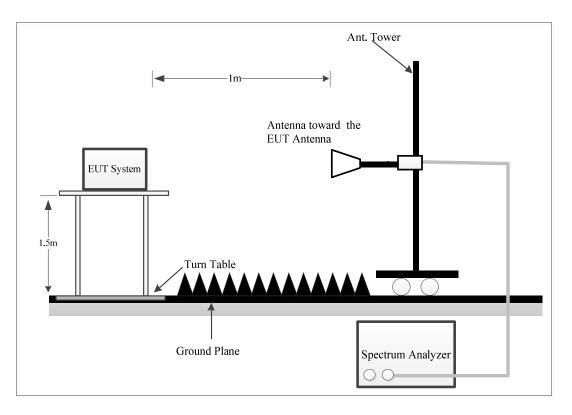
Place the measurement antenna at a measurement distance that is in the far-field of the measurement antenna, in the far-field of the EUT antenna. The EIRP test was performed at 1m distance, which was larger than the minimum test distance, please refer to section 4.2.4 for more detail.
