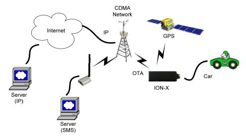
This product will be designed based on the VIA CBP8.2 CDMA 1X 800M&1900M Baseband chipset, which includes GPS functionality, ARM CPU and CDMA protocol. This baseband external connection 64Mb serial flash, CDMA 800M/1900M/GPS RF Transceiver, and RF Front end circuit.
